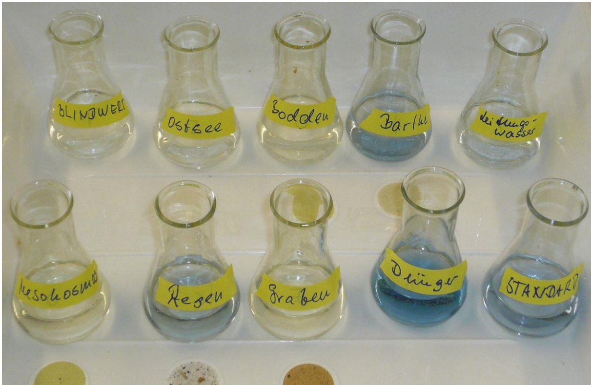
Figure 5.2.3-1 Erlenmeyer flasks with different phosphate-containing and phosphate-free samples (molybdenum blue, standard= 5 \mu\text{M l}^{-1} ). Filters are strongly discoloured partly by the filtrated seston.
