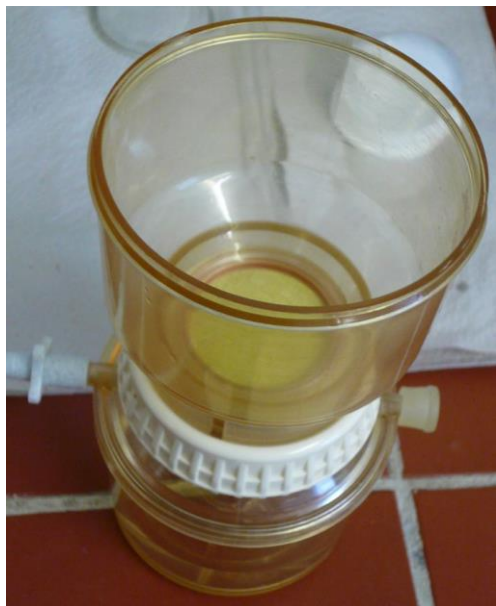
Figure 5.2.3-2 a Filtration trestle with filter (GF 6, 47 mm). Connection to pump (-200 mbar pressure) on the left.
